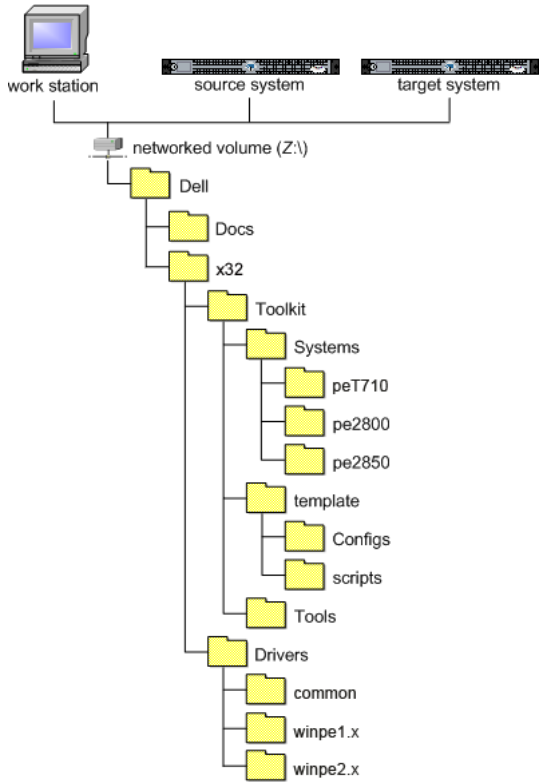
Figure 3-2. DTK System-Specific File Structure
